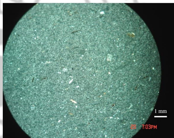
Figure 3: Clinoptilolite, opal-CT and mica minerals are seen in the microscopic appearance of the thin section of Gordes zeolite (A CPL and B PPL).
