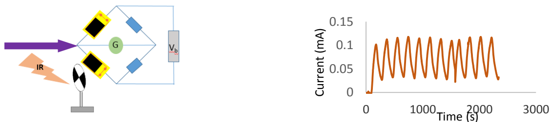
Fig. 1 A schematic view of the photoconductivity properties of PPy-CdS nano-composite film.
