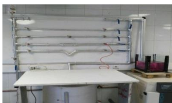
Fig. 1 one of Pressure drop measuring device by Different channels of fluid flow.
