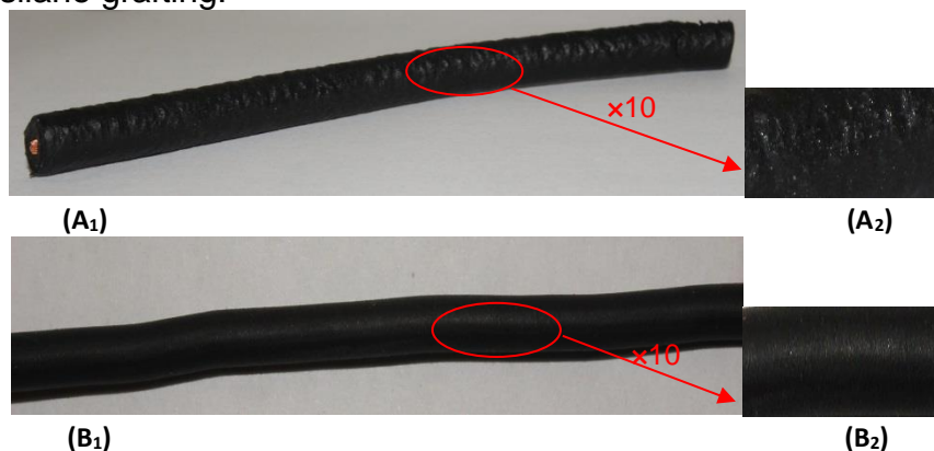
Figure 1. Effect of pre-crosslinking of silane grafted compound on the product appearance. Monosil process (A 1 and A 2 ) and Sioplas process (B 1 and B 2 ). A 1 and B 1 have a resolution of 5184×1114 pixels; A 2 and B 2 have a resolution of 295×181 pixels.
