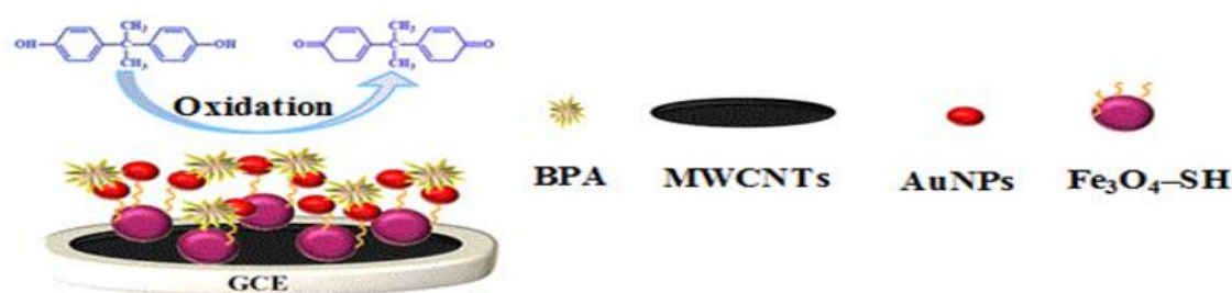
Fig. 1 Schematic of electrochemical bisphenol A sensor.
