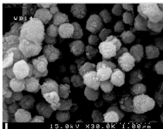
Fig 2. SEM image of \alpha -Fe 2 O 3 -NP
