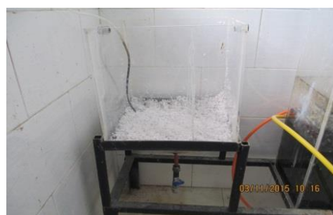
Figure2. Active reactor with ground zeolite
