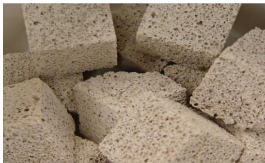
Figure 1: SiO 2 Support ultralight with high porosity
