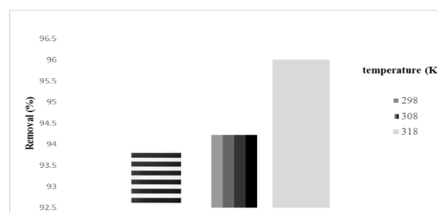
Fig.6: Effect of temperature on dye removal ([C 0 ]: 20 mg/L, adsorbent dosage: 0.3 g/L).
