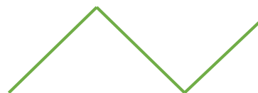
Fig 6-1: repeat unit for chiral vector (6, 0) (zigzag)
