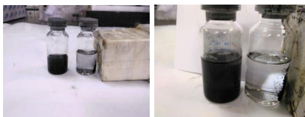
Fig.2. Photograph of the dispersed composite in the model Fuel and separation by magnet.
