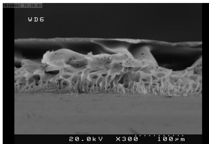
Fig.2: SEM cross-sections of PES/PVDF membranes
