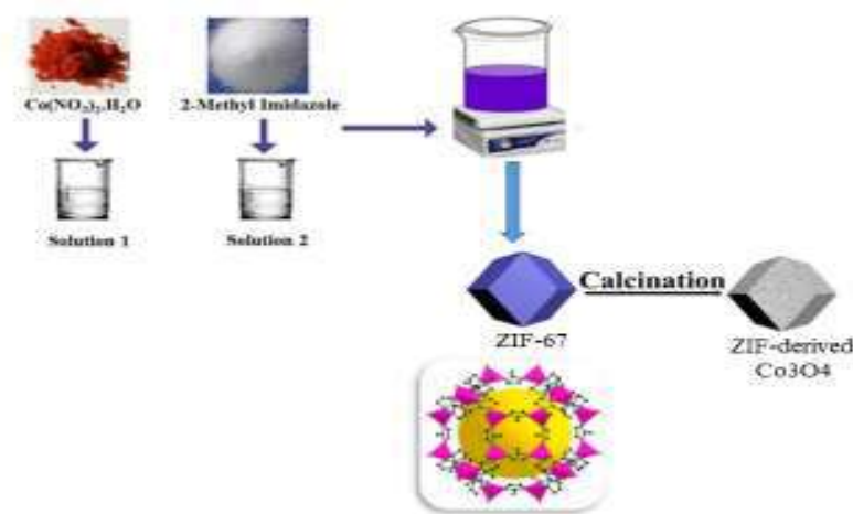
Scheme1: ZIF-67 Derived Hollow Structured Co 3 O 4 Nanocatalysts.
