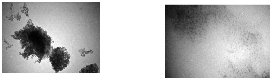
Fig. 1 TEM images of the a) IO@PEG@SiO 2 and b) IO@OA nanoparticles
