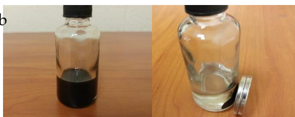
Figure 1: MoS 2 /Fe 3 S 4 dispersed inside the model oil and b) separated from the model oil after seconds of exposure to an external magnet.
