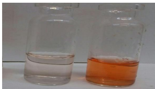
Scheme 1. Degradation of Congo red dye (20 ppm) using synthesized photocatalyst (0.02 g) in 70 minute under visible irradiation.
