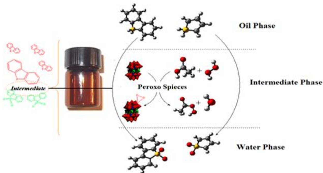
Scheme 1. Mechanism oxidation desulfurization of simulated gas oil
