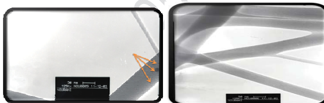
Fig 2: TEM micrographs of nanofibers obtained from electrospinning of CS/PEO solution in 70 % acetic acid at ratio of 70/30 and the presence of nanoparticles.
