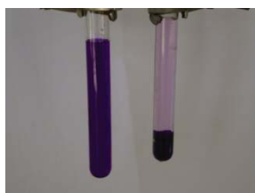
Figure 2: The Crystal violet solution before (left) and after adsorption (right).
