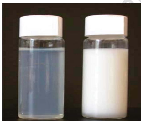
Fig. 1.a) Picture of a Nanoemulsion (left) and a Macroemulsion (right); b) Pseudo-ternary phase diagrams for IPM, Tween 80/ Isobutanol ratio of 2.4/1, Water
