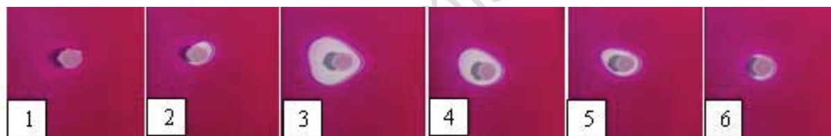
Figure 1. Snapshot of one cycle of the oscillation of the twinkling star with time. The purple and colorless phases contain lower and higher concentrations of the \text{OH}^- ion, respectively.
