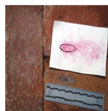
Fig. 4. Lead Splash as a Result of a Low Incident Angle Impact and Ricochet
