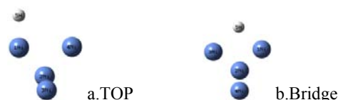
Fig.2. Schematic illustration of H adsorption on Ni 4 (001) cluster for three sites.
