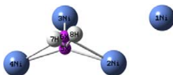
Figure 2 - Schematic illustration of H 2 adsorption on Ni 4 (001) cluster for threefold site. As can be seen, 1.2 Å distance of surface had the most negative energy and is more stable.
