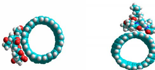
Figure 1- MD simulation snapshots (cross-sectional view) of the wrapping of a CNT (10,10) by poly vinyl pyrrolidone (Left side) and poly vinyl acetate (Right side).
