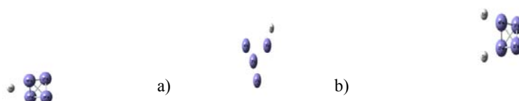
Figure 2: The adsorption of hydrogen atom on two different sites top (a) and bridge (b) in different surface coverage for Fe.
